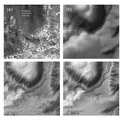
Figure 2. Comparative images of various topographic data sets: (a) 1/5000 aerial topographic map, (b) 40 m digital elevation model (DEM), (c) 1 m × 1 m LiDAR digital surface model (DSM), which includes the presence of vegetation, and (d) 1 m × 1 m LiDAR digital terrain model (DTM) without vegetation.
