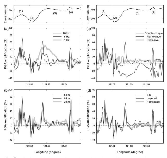
**Figure 9.** Effects due to variations in (a) source frequency, (b) source depth, (c) input wave-field type, and (d) subsurface structure by analyzing the relative change in PGA along profile A-A' in Figure 8a. The upper panels show the related cross section of the LiDAR DTM. Four specific locations are labeled by numbers along the profile.
