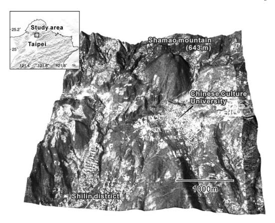
Figure 1. LiDAR 3D digital map of northern Taiwan. A 1/5000 aerial picture is mapped on the 1 m × 1 m LiDAR digital terrain model. The steep peak of Shamao Mountain, the high population density at the Chinese Culture University, and the Shilin district are the most striking features in the region.
