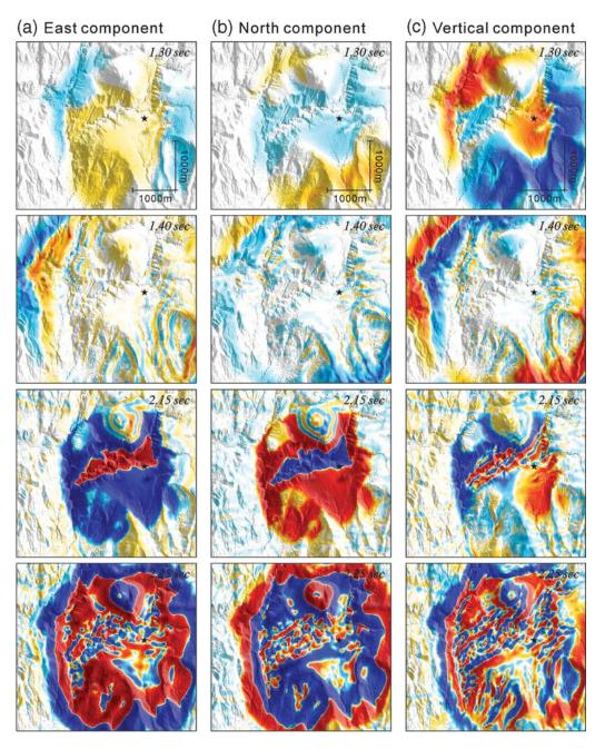
**Figure 4** Snapshots of the three components of the wave field for a simulation of a hypothetical double-couple source located beneath the study area at a depth of 4.92 km: (a) east component, (b) north component, and (c) vertical component. Warm colors indicate positive values and cold colors indicate negative values. The wavefronts are significantly distorted. They are reflected and scattered by steep topography, especially the horizontal components.
