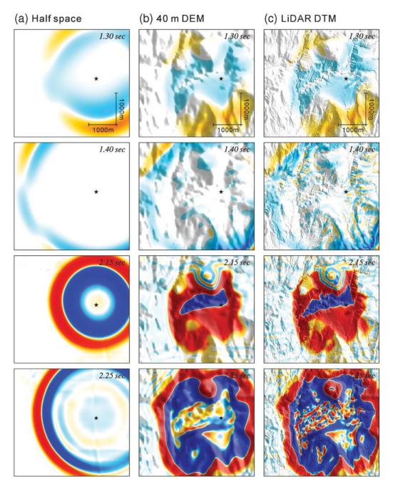
**Figure 5.** Snapshots of the north component of the wave field for three models: (a) 3D wave-speed model with a flat ground surface, (b) 3D wave-speed model with 40 m DEM topography, and (c) 3D wave-speed model incorporating LiDAR DTM. Warm colors indicate positive values and cold colors indicate negative values. The epicenter of the double-couple source is represented by a star.
