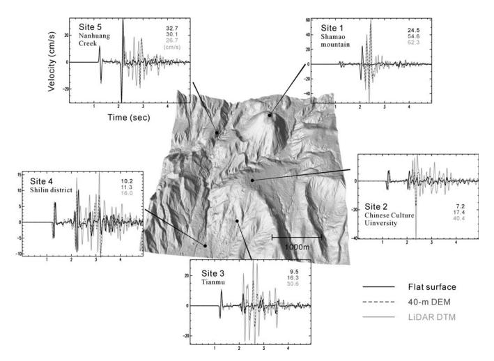
**Figure 7.** Comparison between LiDAR DTM, 40 m DEM, and flat surface synthetic waveforms at five different sites. We show the vertical component of the velocity vector, band-pass filtered between 0.1 and 10 Hz. Gray lines show the LiDAR DTM synthetic seismograms, dashed lines show the 40 m DEM synthetic seismograms, and black lines are the flat surface synthetic seismograms. Peak velocities determined for the three models are shown in the right-hand side of the figure.
