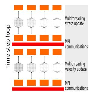
Figure 5. Two-level parallelism with four MPI processes. Each MPI task creates a pool of threads for the update of velocity and stress unknowns.
