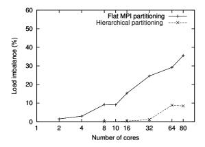
Figure 6. Load balancing comparison between a pure MPI approach and a mixed approach: the hybrid methodology is clearly superior.
