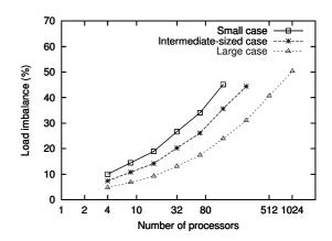
Figure 3. Theoretical load imbalance for a finite-difference parallel simulation and impact of CPU-costly boundary conditions. We have considered three different grid sizes.
