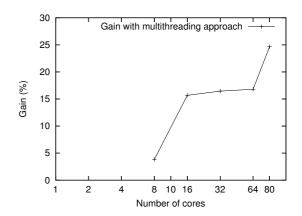
Figure 7. Gain in terms of elapsed time for the French Riviera example on 80 CPUs. The comparison with the pure MPI approach shows a maximum 25 % reduction of computation time.
