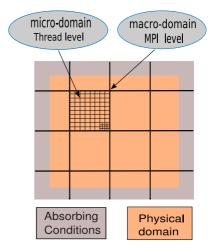
Figure 4. Top view - Hybrid partitioning of our 3D computational domain. Each MPI macro-domain creates a hierarchy of microdomains.
