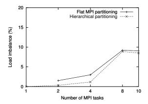
Figure 8. Comparison of pure MPI and hybrid partitioning behaviour in terms of loadbalancing at the macro-domain level.
